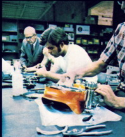
Band masks are checked and double-checked during every stage of assembly... then checked again prior to packaging. Each is water tested for leaks and for proper communications. Upon completion, each is used in a test dive to assure our inspectors there are no air leaks, the mask seals properly, and that the installed communication equipment is functioning properly.
