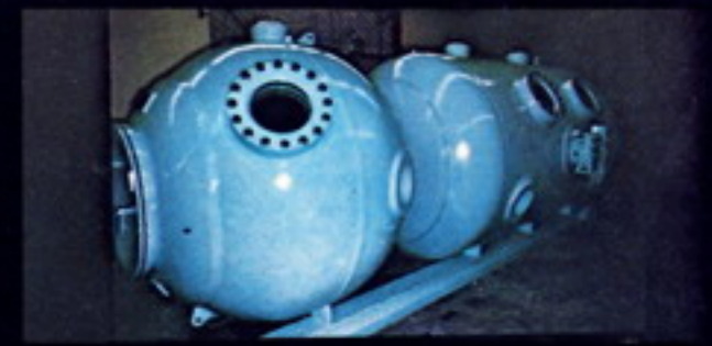
New hyperbaric chamber tests men and equipment from simulated altitudes of 60,000 feet to depths of 1,650 feet—giving U. S. Divers Co. one of the most complete test facilities in the world.
